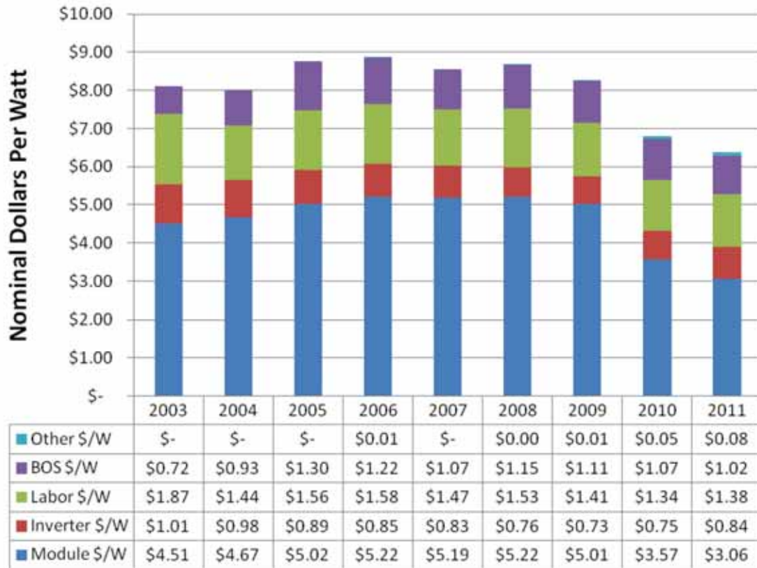
Figure 9. PV System Prices by Component in the NYSERDA Upfront Incentive Program Database 2003-2011 37
